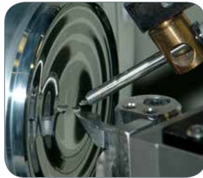
Rotation-symmetric multiple aspherical surface, aluminium.
