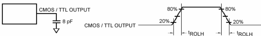
Figure 9. Receiver LVTTTL/CMOS Output Load and Transition Times
