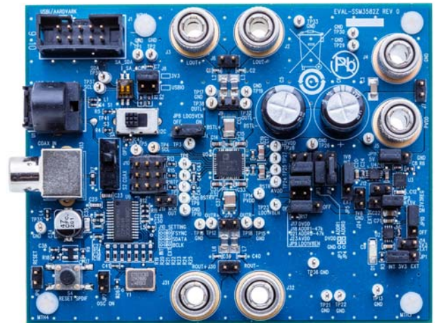
Figure 1. EVAL-SSM3582Z Evaluation Board, Top View
