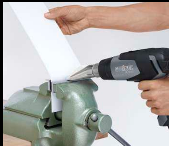
Using heat for getting plastic into exactly the right shape.
