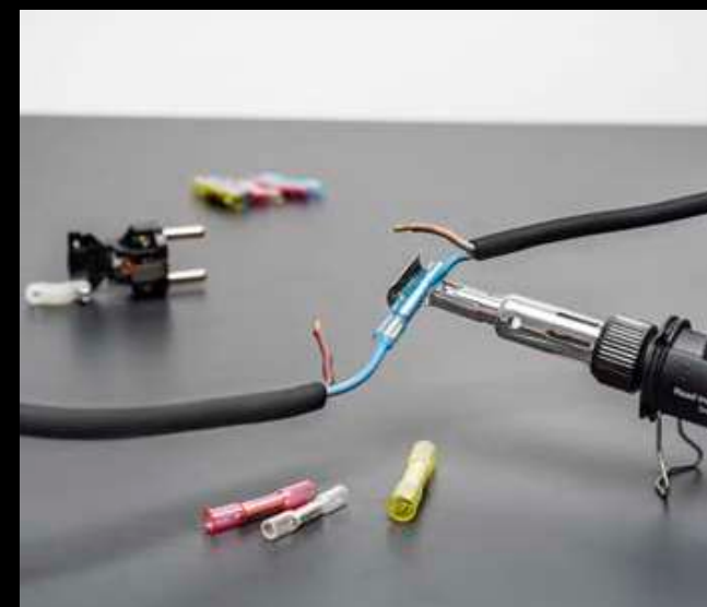
Create an even seal on solder sleeves
